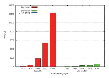
Fig. 17. TLS/SSL VS Our proposed protocol: Total computational workload.
