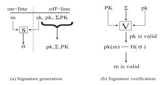
Fig. 12. The  $\lambda_{LAKE}$  authenticator: (a) signature generation and (b) signature verification.
