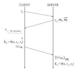
Fig. 2. A sketch of the TLS/SSL handshake.
