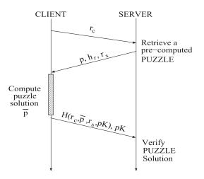
Fig. 19. Avoiding DoS/dDoS with puzzles: the server asks the client for a puzzle solution before initiating the key-establishing protocol.
