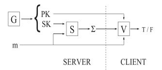
Fig. 3. Signing and verification of a message with an ordinary signature scheme.
