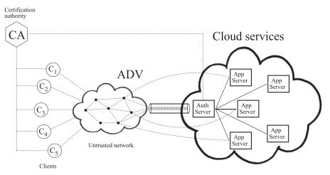
Fig. 1. Reference scenario. Clients need to be granted by the authentication server (Auth Server) in order to subsequently access the application servers (App Server).
